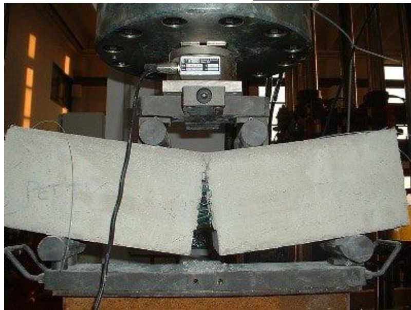
Brittle Concrete beam ( not favorite )
