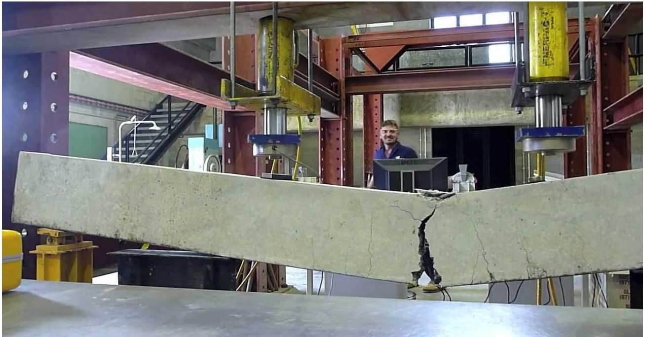
Tension failure of beam ( permitted in ACI Code)
